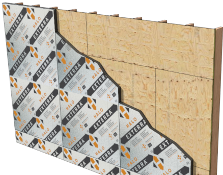
Offset horizontal and vertical joints between HALO Exterra and wood sheathing when possible.
