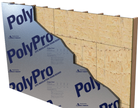
Offset horizontal and vertical joints between PolyPro and wood sheathing when possible.
